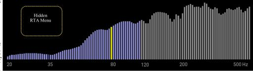
Conversion of the audio signal data collected by the device's on board microphone, are turned in to visual representations and displayed in graph form. This type of instrument is very useful to see the effects of augmenting the bass detail in your system. The response speed of the RTA display is limited only by the speed of your device.
