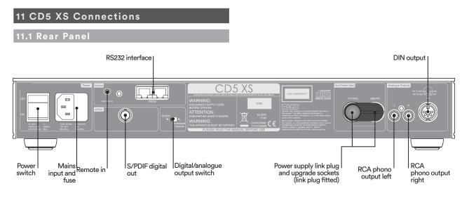
**Note:** The power supply link plug should be fitted unless an external upgrade power supply is in use.
