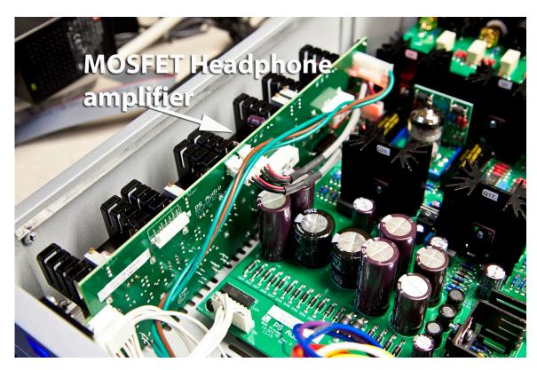
When you insert the headphone jack into the front panel headphone connector, the preamplifier will automatically disconnect the preamplifier outputs. This permits the use of headphones without also having the loudspeakers play at the same time.
