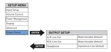
The Output section of the Setup menu lets you configure the outputs.
