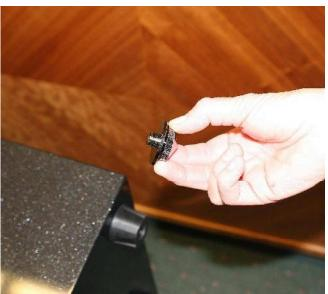
**Step 6 -**Place the leveling washer onto the cone.
