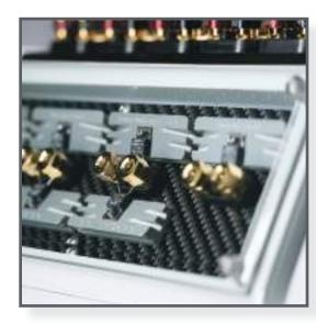
Woofer Module of your Chronosonic XVX, you may gain access to the resistor plate. These resistors serve several functions.
