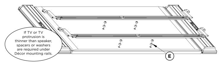
4. Take additional TV rails included in separately purchased TV wall Mount Kit and place onto back of TV overtop of attached speaker rail assemblies.
