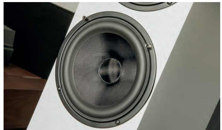
Like the midwoofer, the woofer as well features a cone made of woven glass fibre. Two of the mounting screws - like those of the midwoofer - are designed as protruding pins. They are used to fix the detachable front grille. This integrative measure allows for the baffle to remain free of visually disturbing elements.
