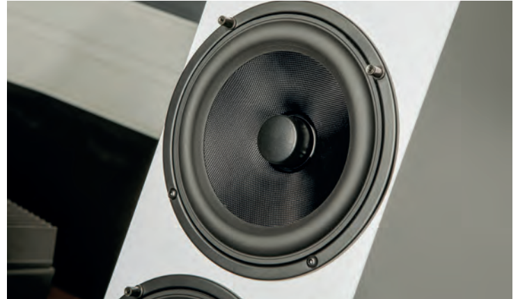
As the midwoofer takes on the heaviest job, it features a phase plug for heat dissipation. To keep the driver securely fixed and to prevent vibration transfer into the cabinet, the mounting screws use neoprene dowels as counterparts.
