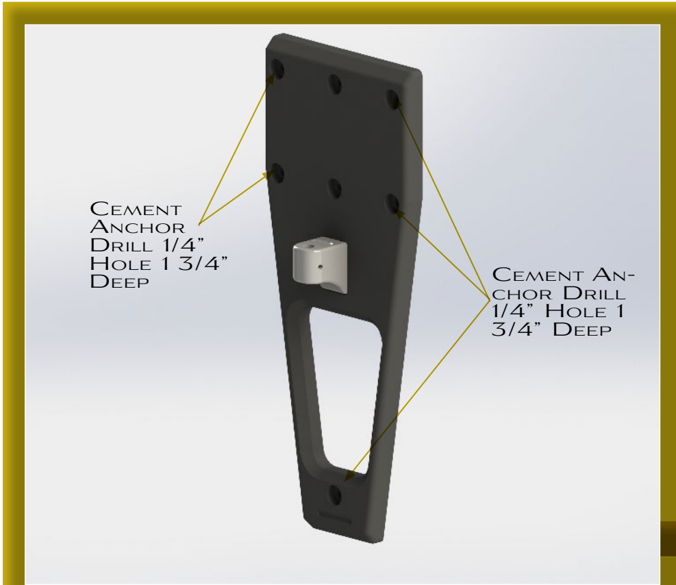
FIGURE 3—MOUNTING LOCATIONS FOR FOR A CONCRETE WALL
