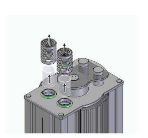
Loosen the tube covers by turning them counterclockwise and then remove them upwards.
