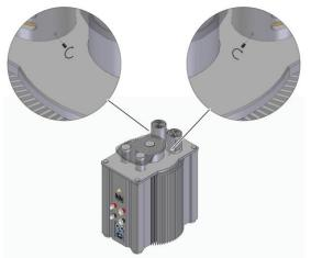
Finally, insert and tighten the grounding screws.
