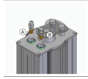
Insert tubes as shown (observe marking on tube socket).
