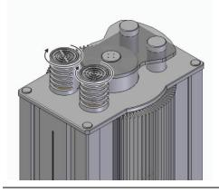
Tighten the tube cover clockwise.
