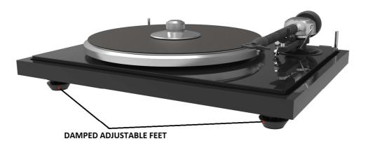
Three precision adjustable damped feet are mounted under the turntable for leveling the turntable. Once the turntable is in final position, put the supplied spirit level on the sub-chassis, and then level the turntable by screwing or unscrewing the feet as needed. It is advisable to check level from several positions on the subchassis.
