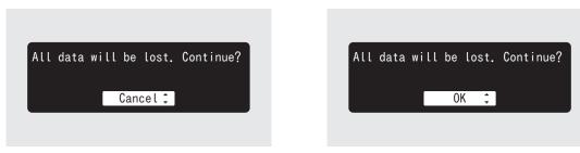
Move the cursor by pressing the Up button ( $\wedge$ ) or the Down button ( $\vee$ ), then press the Menu/Enter button ( $\sqsubseteq$ ) to make a selection.
