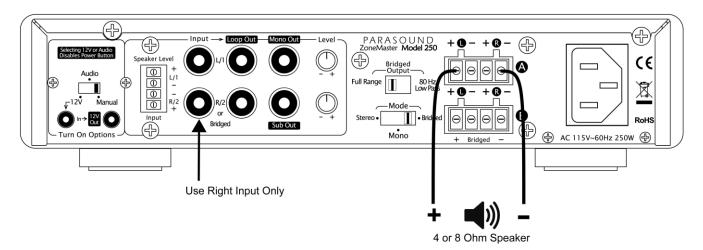
**Two Speakers:** Connect the speaker's positive (+) terminal to the **L+** on the **A** output. Connect the speaker's negative (-) terminal to the **R -** on the A output. Do the same for the second speaker on the **B** output. Use only the Right input jack. Each speaker must be 8 ohms. Both speaker will play the same mono signal. Both speaker output A and speaker output B use the same connection method even though the rear panel only shows the bridged polarity under the B output.
