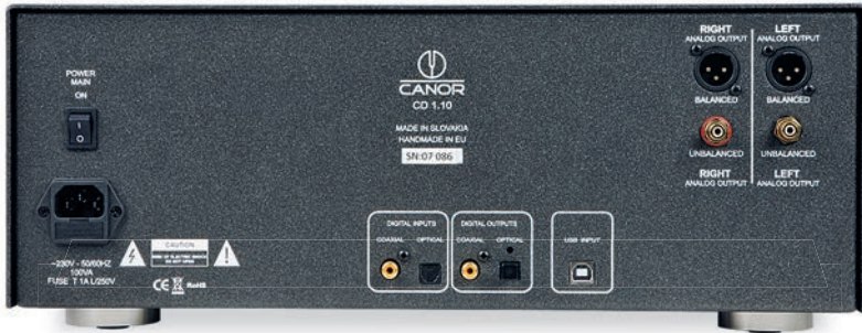
ABOVE: Rear panel has coaxial and optical digital inputs and outs plus USB digital in, and RCA and balanced XLR line outputs. IEC mains socket sits below power switch
