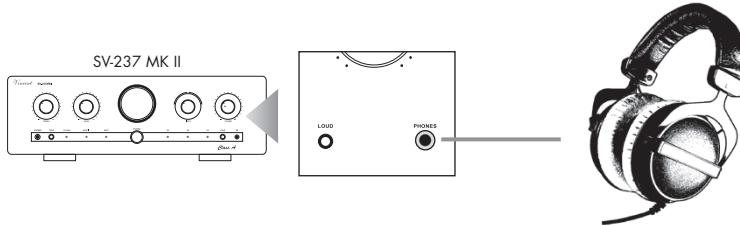
By doing this, the loudspeakers are switched off. All headphones with an impedance of between 32 Ohm and 600 Ohm may be used. Unsuitable headphones with too low impedance may damage the amplifier or produce such unexpectedly loud volume that your hearing may be damaged. The volume (5)(25) should be reduced for safety reasons before a set of phones is connected.
