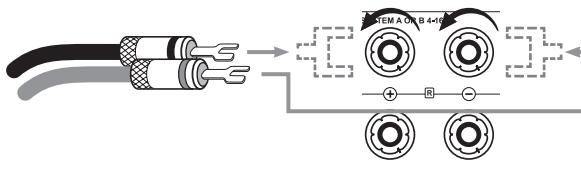
If no connector is to be used, remove approximately 1 cm length of insulation from each end of the speaker wire. Twist the braid in order to avoid short circuits. Turn the fastener on the loudspeaker terminal counter clockwise to loosen it and introduce the bare wire end into the exposed connector hole. Then turn the fastener clockwise so that the wire is firmly clamped. Make sure the connection is pretty tight.
