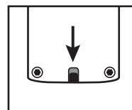
2. Remove the optionally used battery and correctly insert the new button cell, as schematically shown in the battery compartment.
