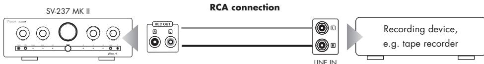
Connect this signal output to the signal input ("LINE IN", "TAPE IN" or "REC IN") on the recording appliance using RCA cables. Please note that some recording equipment can have a slightly detrimental effect on the audio signal quality. Some recording devices have rather low input impedance, which can slightly alter the input signal voltage. For maximal music enjoyment we recommend that you connect to the "REC" terminal only for as long as the recording is actually being made.
