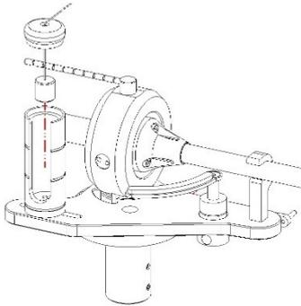
Put the anti-skating weight with its cap and string attached into the housing as seen in the above left picture. Then fix the soft eye of the string on the anti-skating lever. Please adjust it according to the above right picture.
