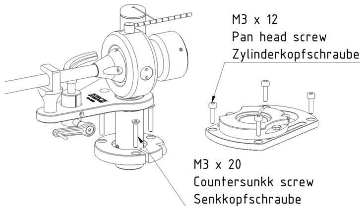
Take the provided either 3x M3x20 countersunk screws or 4x pan head screws M3x12 and insert them into the marked appropriate holes of the mounting flange (see picture above).
