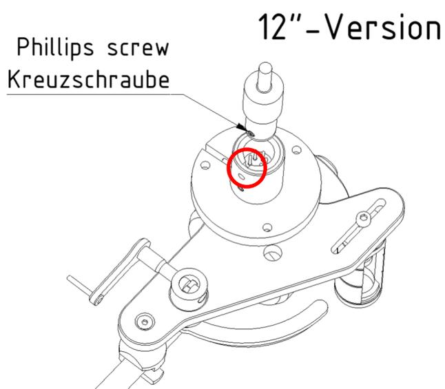
Looking from the bottom of your TA-1000 Neo you can see the 5 pin plug and its alignment. The connector has a small Phillips screw on its cylinder. This screw must face towards the cartridge when being inserted in the plug. Please insert the connector carefully; otherwise the pins might be damaged.
