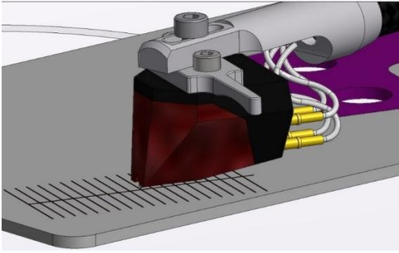
Lift down the cartridge and place the diamond tip of the cartridge on the reference point of the adjustment template and make sure that the edges of the cartridge are parallel to the marking lines printed on the template.
