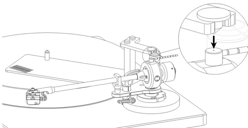
Put the template on the platter using the bore for the desired tonearm length. Move the tonearm forward or backward, so that the centering fits into the drilled marking on top of the tonearm. Tighten the tonearm with either its 3 screws (Rega base mount) or its 2 hexagon head screws (SME base mount) in the round mounting flange, when the position fits. This ensures the correct angle and distance of the template for adjusting the cartridge.
