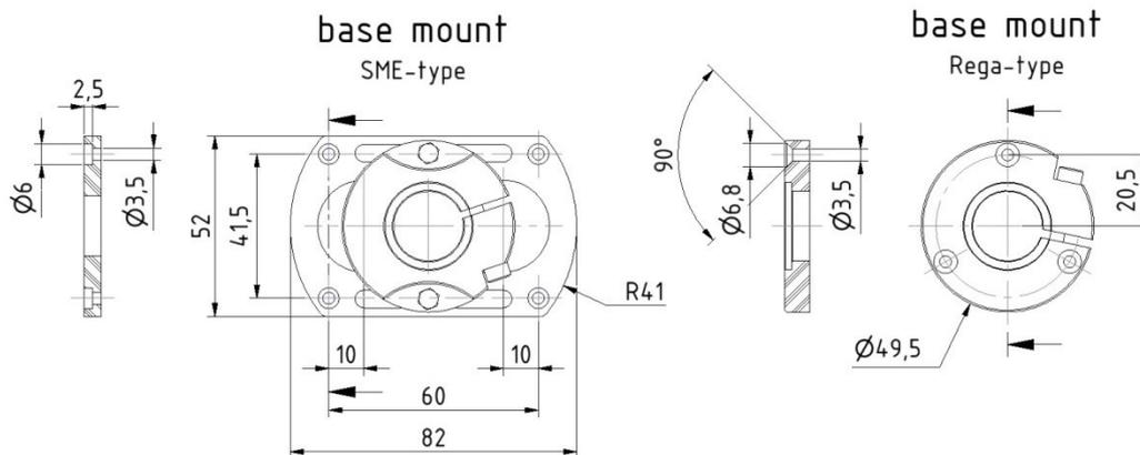
To mount the **TA-1000 Neo** tonearm with the Rega-type base mount your turntable needs to have a 24mm thru hole combined with 3x M3 threads around it at a Radius of 20.5 mm.
