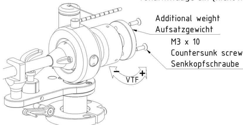
After adjusting the VTF please tighten at least one the 3 screws in the counterweight.
