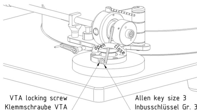
Adjust the arm height with cartridge fitted, so that the arm tube is either parallel or slightly lower at the front end.
