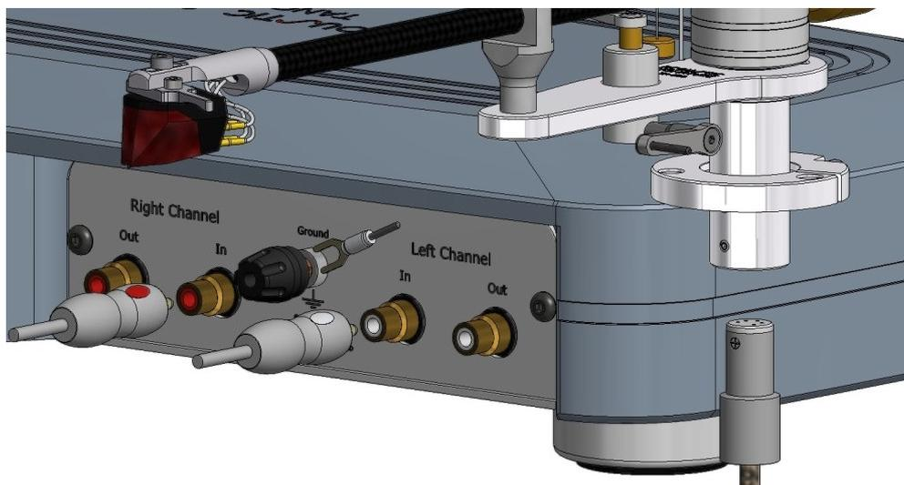
Finally connect the RCA-connectors and the ground connector to the matching input plugs of your phono pre-amplifier
