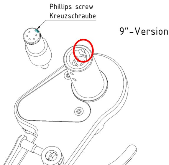
Looking from the bottom of your **TA-7000 Neo** you can see the 5-pin plug and its alignment. The connector has a small Phillips screw on its cylinder. This screw must face towards the cartridge when being inserted in the plug. Please insert the connector carefully; otherwise, the pins might be damaged.
