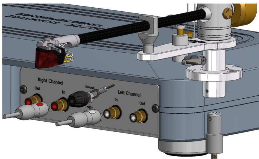
Finally connect the RCA-connectors and the ground connector to the matching input plugs of your phono pre-amplifier
