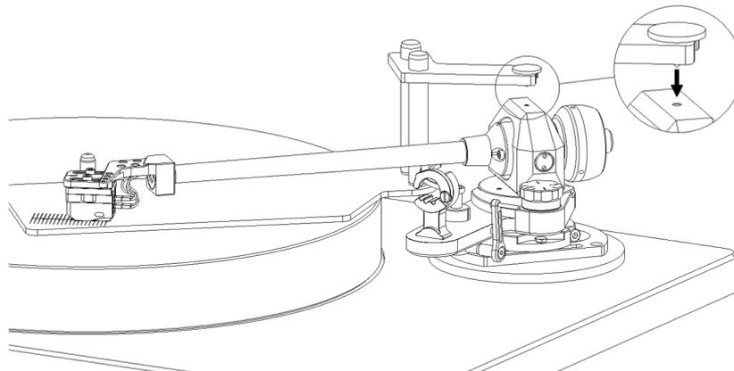
Put the template on the platter using the bore for the desired tonearm length. Move the tonearm forward or backward, so that the centering fits into the drilled marking on top of the tonearm. Tighten the tonearm with either its 3 screws (Rega base mount) or its 2 hexagon head screws (SME base mount) in the round mounting flange, when the position fits. This ensures the correct angle and distance of the template for adjusting the cartridge.
