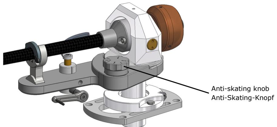
To adjust the Anti-skating use the Anti-skating adjustment knob and adjust the correct value by slowly turning the knob, starting with 0.
