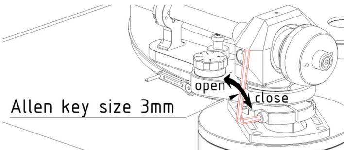
Adjust the arm height with cartridge fitted, so that the arm tube is either parallel or slightly lower at the front end.
