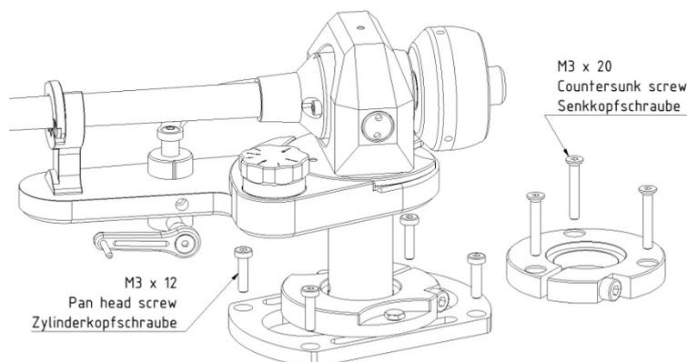
Take the provided either 3x M3x20 countersunk screws or 4x pan head screws M3x12 and insert them into the marked appropriate holes of the mounting flange (see picture above).
