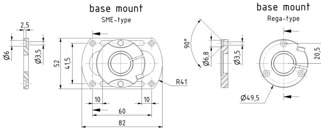
To mount the **TA-7000 Neo** tonearm with the Rega-type base mount your turntable needs to have a 24mm thru hole combined with 3x M3 threads around it at a Radius of 20.5 mm.
