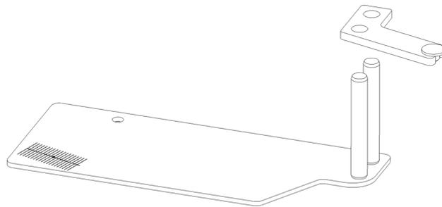
This is done by using the provided adjustment template. Take the two parts of the template and assemble it, as shown in the picture above, and place it on the platter.
