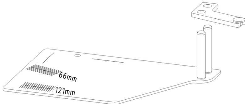
This is done by using the provided adjustment template. Take the two parts of the template and assemble it, as shown in the picture above, and place it on the platter.
