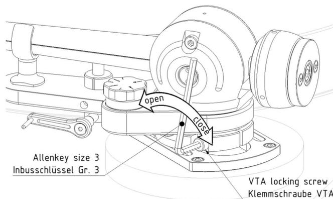
Adjust the arm height with cartridge fitted, so that the arm tube is either parallel or slightly lower at the front end.
