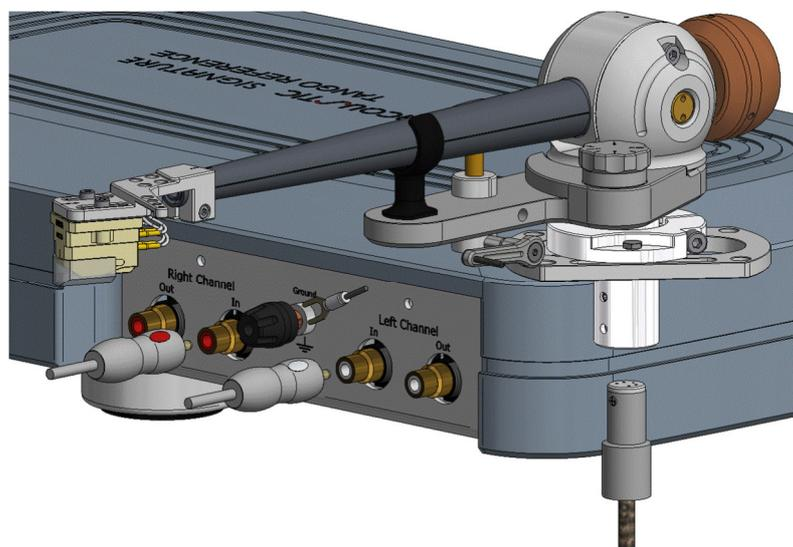
Finally connect the RCA-connectors and the ground connector to the matching input plugs of your phono pre-amplifier
