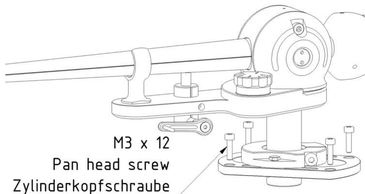
Take the provided 4x pan head screws M3x12 and insert them into the marked appropriate holes of the mounting flange (see picture above). Use the provided Allen key to tighten the screws. To get easier access to the holes, it might be helpful to turn the complete tonearm within the mounting flange so the holes are free. Or you can take out the tonearm and assemble the mounting flange first.
