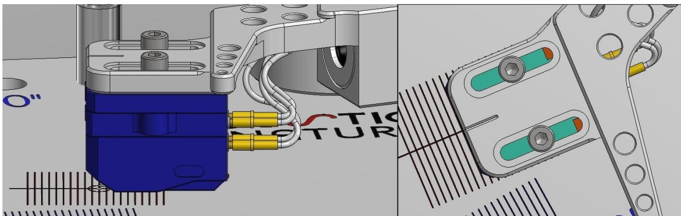
Lift down the cartridge and place the diamond tip of the cartridge on the reference point of the adjustment template and make sure that the edges of the cartridge are parallel to the marking lines printed on the template.
