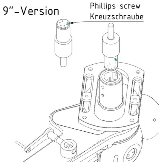
Looking from the bottom of your **TA-9000 Neo** you can see the 5 pin plug and its alignment. The connector has a small Phillips screw on its cylinder. This screw must face towards the cartridge when being inserted in the plug. Please insert the connector carefully; otherwise the pins might be damaged.
