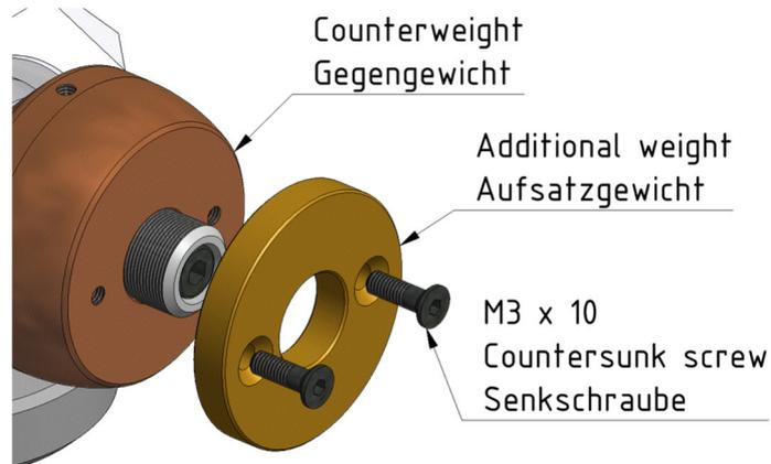
After adjusting the VTF please tighten at least one the 3 screws in the counterweight.
