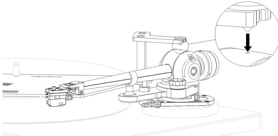
Put the template with its bore onto the record centerpin and the surface of the platter. Move the tonearm forward or backward, so that the centering fits into the drilled marking on top of the tonearm. Tighten the tonearm with its 2 hexagon head screws in the base mount (in the round mounting flange), when the position fits. This ensures the correct angle and distance of the template for adjusting the cartridge.
