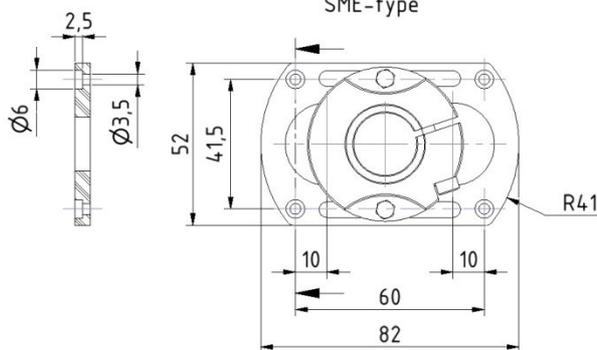
To mount the **TA-9000 Neo** tonearm with the Rega-type base mount your turntable needs to have a 24mm thru hole combined with 3x M3 threads around it at a Radius of 20.5 mm.
