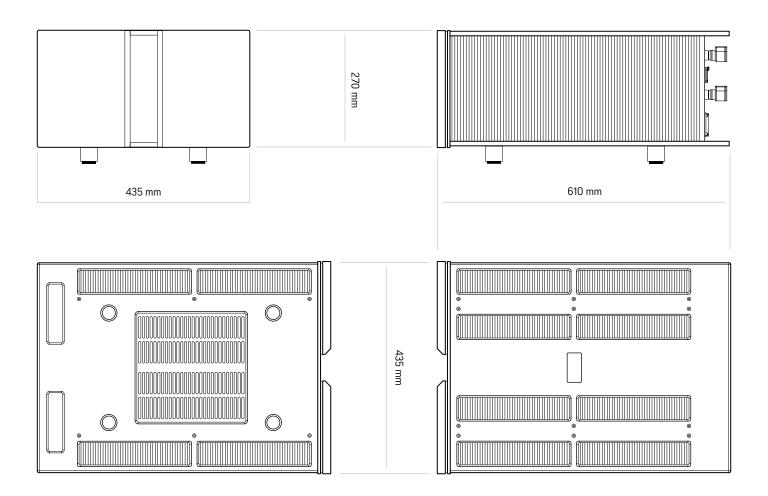
Material: Aluminium for body parts and heat sinks Dimensions (H x W x D): 270 x 435 x 610 (mm) Amplifier weight: 65kg for each amplifier (please note there are 2) PSU weight: 85kg for each PSU (please note there are 2)
