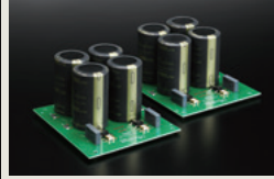
Cumulative 80,000µF filtering capacitors
