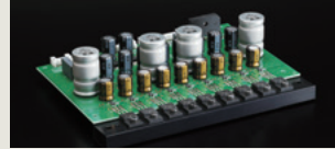
Low noise power supply circuits
