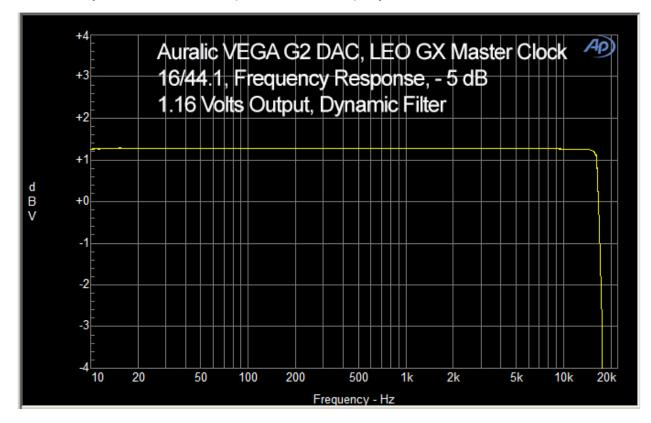
With the Dynamic filter, the response rolls off rapidly above 16 kHz.
