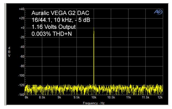
In the spectrum shown below, I added 496 nSec (nano-seconds) of 1 kHz sine wave jitter to the test signal. The 10 kHz peak still has no side peaks. So, jitter is suppressed by the Auralic VEGA G2, with no LEO GX attached.
