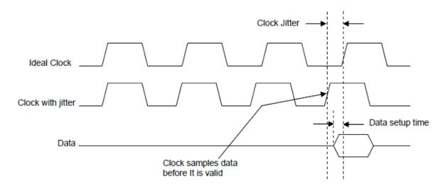
The data hold time is the amount of time that a bit needs to be held in order to be read. If the bit comes too late, again, the microprocessor receives incorrect information.
