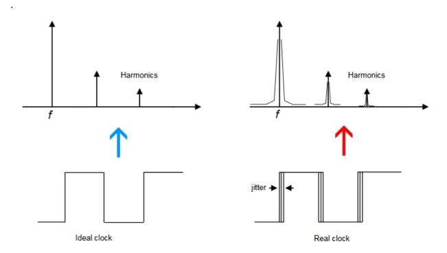
With a perfect (Ideal) clock, the 1's and 0's have no jitter, i.e., the timing is as it should be, shown in the left-hand side of the diagram. Frequencies in the music, and their harmonics, are narrow peaks. With the real world (Real Clock), the 1's and 0's do not arrive exactly when they should, and the frequencies in the music, and their harmonics, appear with widened peaks, especially at the base (right-hand side of the diagram). Some of this is side-band peaks, distorting the music.
