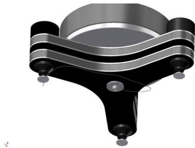
Pic. 3: Grounding the bearing of the Innovation
