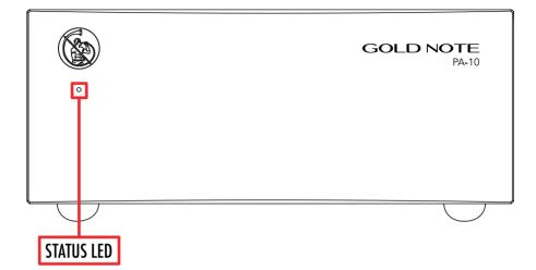
The status led turn blue when the PA-10 is powered.
