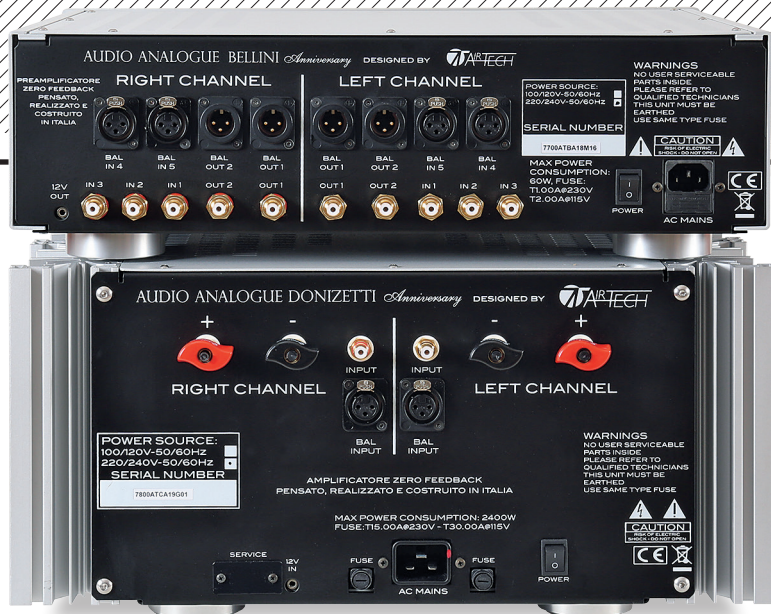
ABOVE: The preamp [top] offers five line ins (three on RCAs and two on XLRs), two tape ins (on RCAs), and four sets of main outputs (on RCAs and XLRs). The power amp [below] has inputs on RCAs and XLRs plus 'wing nut' 4mm cable binding posts
