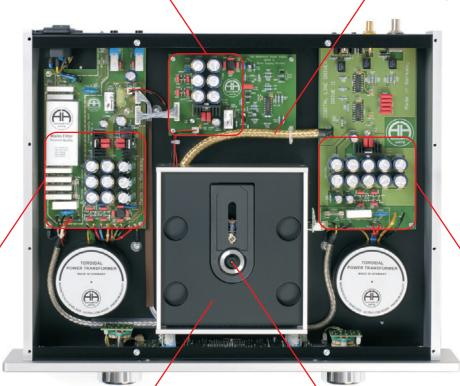
High performance power supply for the digital signal processing with very accurate voltage stabilization made of finest selected components
