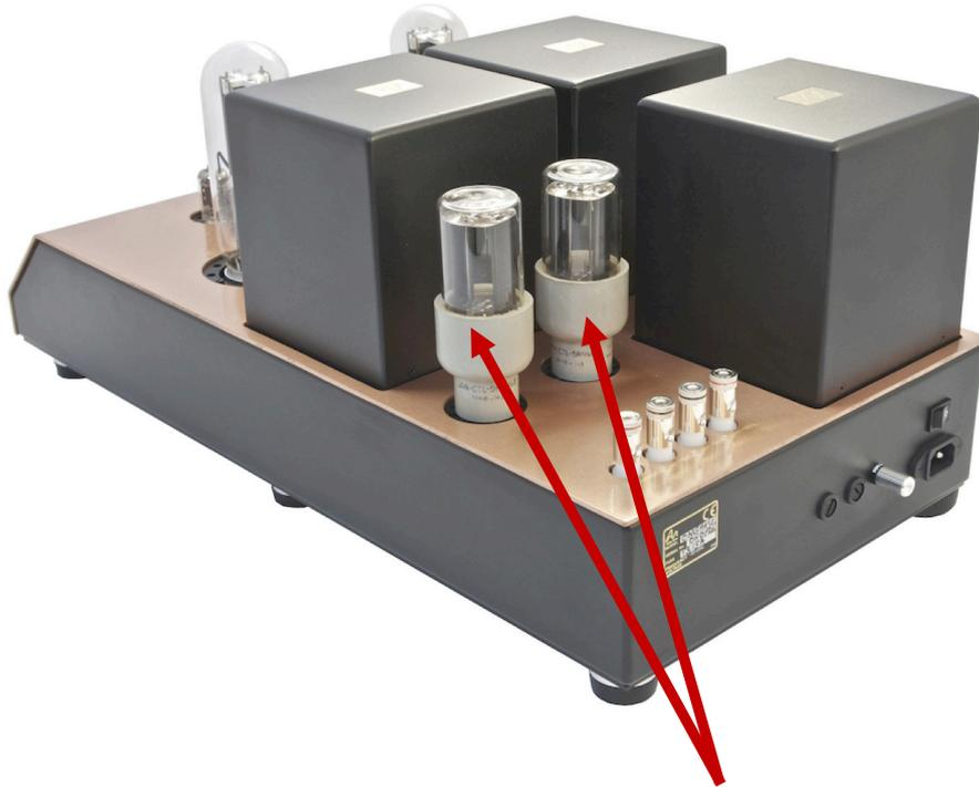
Looking from the back of the amplifier, insert the **5R4WGB** valves into the two empty sockets located on the left, situated between the black rectangular transformer covers and the loudspeaker connection binding posts. Locate the rib on the central pin of the valve and align with the valve base (it can only be inserted one way due to this locating rib) and with gentle but firm pressure insert the valve.
