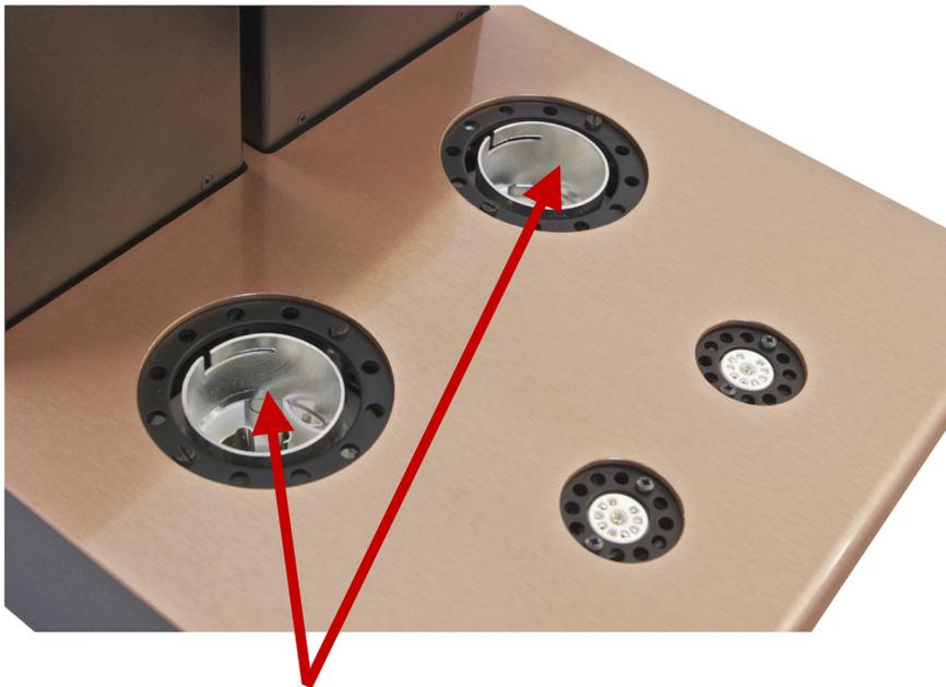
Also examine the **two large apertures** in the top plate of the amplifier, located between the two small valve sockets at the front of the amplifier and the black rectangular transformer covers. These are the insertion points for the VT-4C valves.
