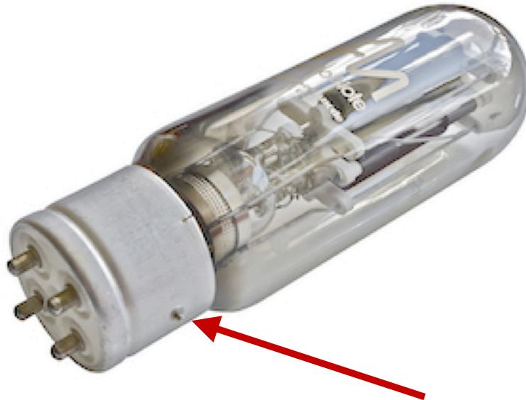
Inspect a VT-4C valve and you will notice that there is a **small 'pin'** protruding from one side of the valve base; this locating pin ensures that the valve can only be correctly inserted into the amplifier in one way.
