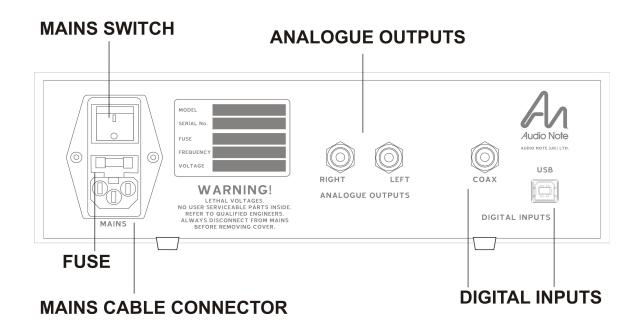
Please ensure that the DACO.1x and any source equipment is switched off before making any connections.
