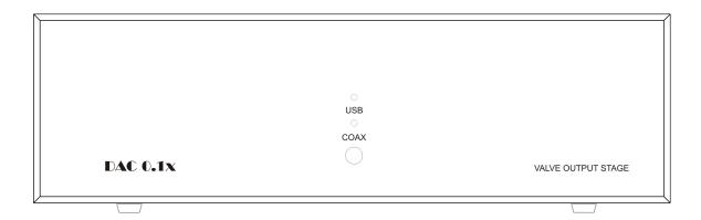
Press button on front panel for short time to select digital input, USB or COAX. Selected input will be indicated by red light.
