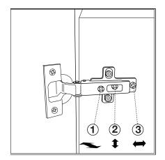
Use the **Phillips Screwdriver T1** supplied to adjust the door hinges:
