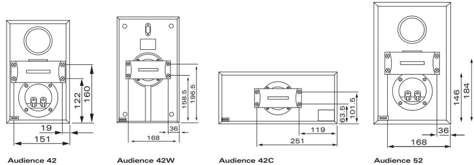
Decide upon the location where the loudspeakers will be mounted and mark the wall at the edges of the longer plate. Also mark the location of the holes in the wall, having firstly checked the vertical positioning with the level.
