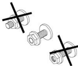
First put the bolt and the plain washer through the slot of the smaller curved plate. Then screw the nut flush onto the bolt, as shown in the picture.
