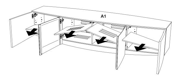
**Step 6 -** With help from another person, carefully lay the **Cabinet A1** on its top (upside down). Attach the base assembly to the bottom of the **Cabinet A1** with **8 Screws H1** as shown using **Hex Wrench T2.** Once all screws have been started, fully tighten all base screws.
