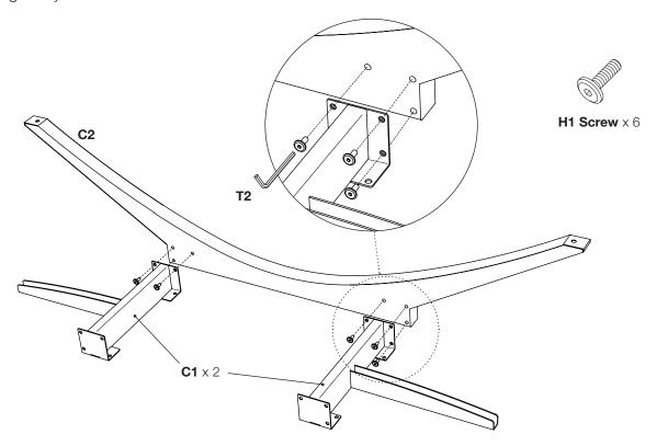
Step 3 - Attach the second Leg Frame C2 to the Sub-frames with 6 screws H1. Do NOT fully tighten yet.
